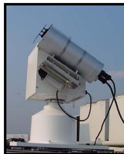
Figure 14: The Kipp & Zonen PGS100 Sun Photometer and a pyrheliosensor mounted below it both shown mounted on a solar tracker [25].
